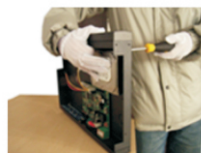
1. Install fixed screw for HDD
